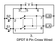
**Duplexing (Cross Wired):** Duplexing models operate the same as alternating relays and when both the Control (S1) and Lag Load (S2) Switches are closed, Load A and Load B energize simultaneously.
